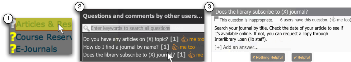
Figure 10.1. Main components of the LemonAid interface in the help mode: (1) a user selects an on-screen label or image highlighted in yellow; (2) the user's selection triggers the retrieval of relevant questions; (3) the user can click on a question to see the answer(s) for that question and indicate whether the answer was helpful or not helpful.
