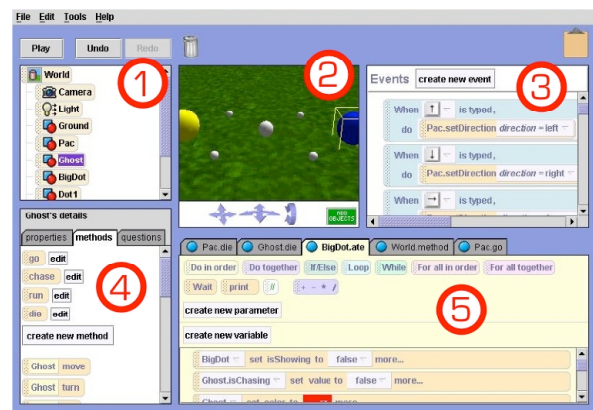
Figure 2. Alice v2.0: (1) objects in the world, (2) the 3D worldview, (3) events, (4) details of the selected object, and (5) the method being edited.
