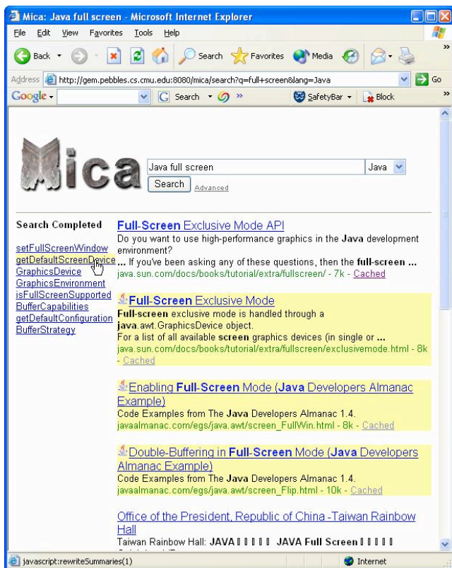
Figure 5. The Mica web application. Mica includes a keyword sidebar on the left, which is generated from Google Web API search results shown on the right. Search result pages containing code are marked with an icon.
