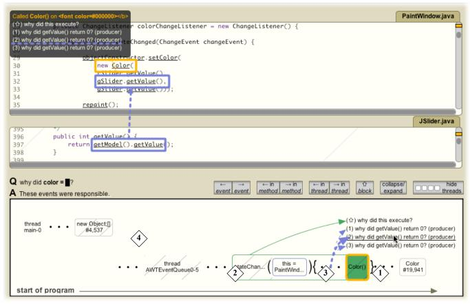
Figure 2. The Whyline's answer to "why did this line's color =  $\blacksquare$ ?", showing (1) the current selection, (2) the use of Java syntax to segment events, (3) two separate threads of execution, and(4) a call container.
