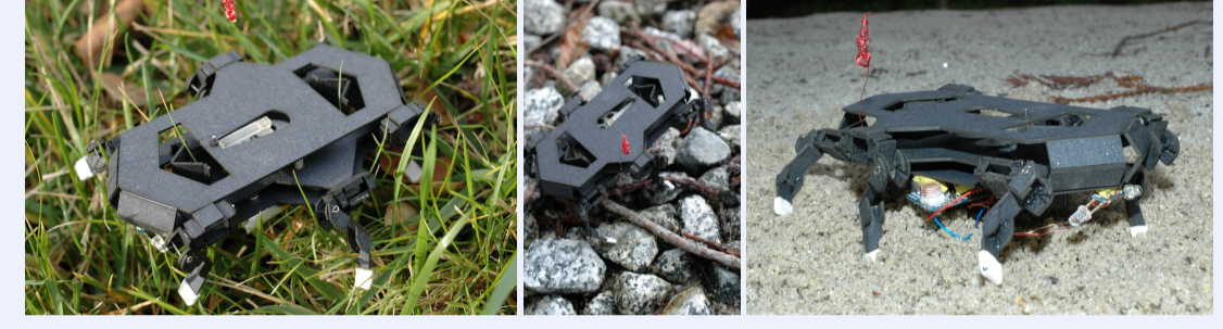
Fig 1: Milliscale hexapedal robot [1] 10cm (L) x 6.5cm (W) x 3.5cm (H) 6mm DC motor; 90 mAhr LiPoly batt. 40 MIPS PIC; 230 Kbps Bluetooth radio Robot dynamics are poorly understood; need hybrid system ID tools to improve design and control
