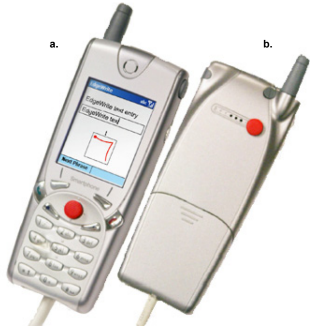
Figure 1. (a) Our Red-E SC1100 Smartphone with an IBM TrackPoint isometric joystick embedded in the front. The phone’s screen shows our text entry software. (b) The same phone showing the other joystick embedded in the back.
