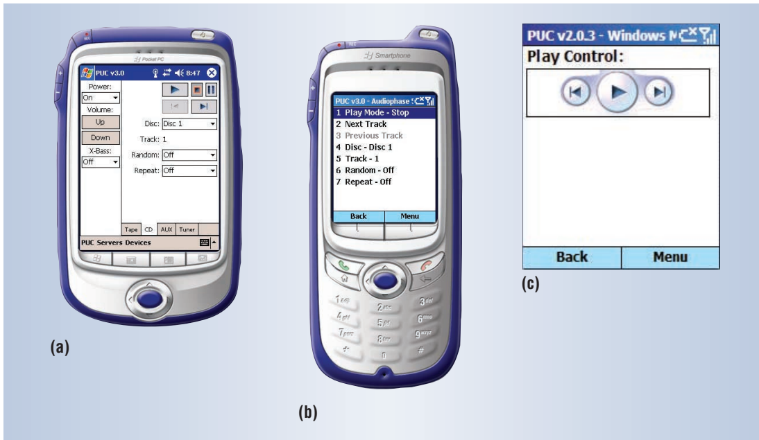
Figure 4. Automatically generated interfaces. (a) An interface for a stereo on a PocketPC and (b) and (c) on a Microsoft SmartPhone cell phone. In (a) and (c), a Smart Template renders the play control buttons.
