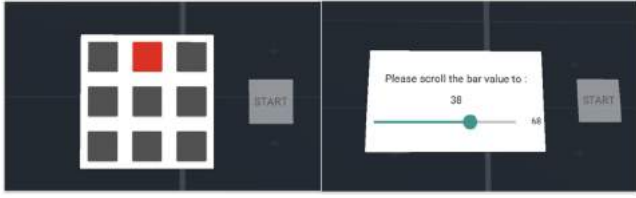
Figure 8: User study tasks. At left is an in-headset view of the button selection task. One of nine buttons randomly turns red for each trial. At right is an in-headset view of the slider manipulation task. The target value is shown on the top of the slider with the bigger font size and bold style. To the right side of the slider is its current value.
