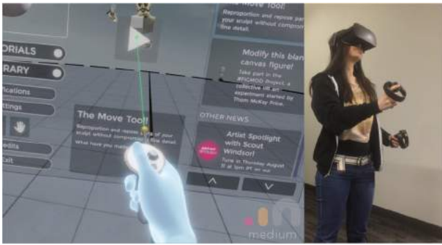
Figure 2: Using Medium [63] for sculpting. The UI is situated within a 3D environment and is activated by a ray cast from the right hand. At left, the in-headset view, and at right, a user making a selection.
