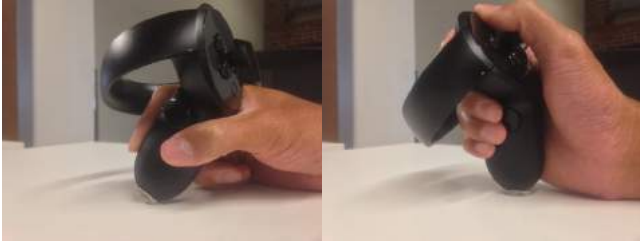
Figure 6: Gripping the Oculus Touch controller. At left is the precision grip we use for table touch. At right is the power grip we use for the world raycast, world touch, and hand touch modalities.
