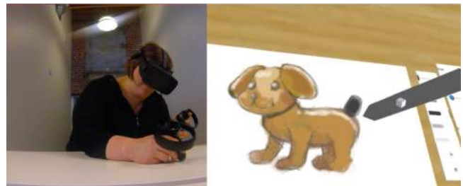
Figure 1: A participant doing 2D sketching in VR using table-top interaction with an office desk. At left is the view of the user at their desk, and at right is the user’s view in the HMD.
