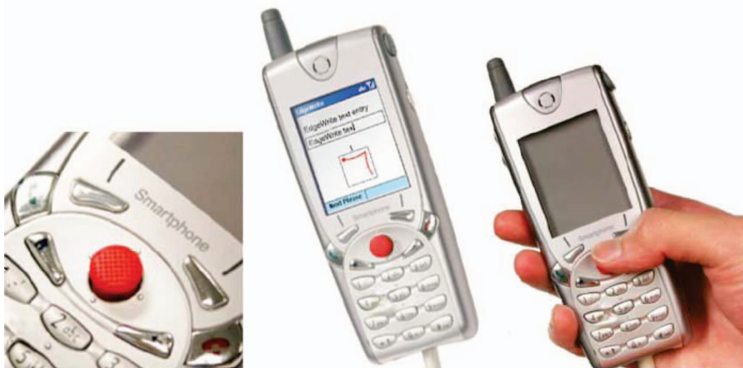
Figure 24. An isometric joystick embedded in a mobile phone. The same software for Trackball EdgeWrite works for the isometric joystick, which can be controlled with the thumb.
