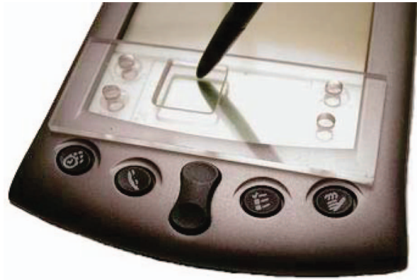
Figure 6. Stylus EdgeWrite on a Palm PDA device. The stylus moves along the edges and into the corners of the square hole, which provides stability for tremulous users.
