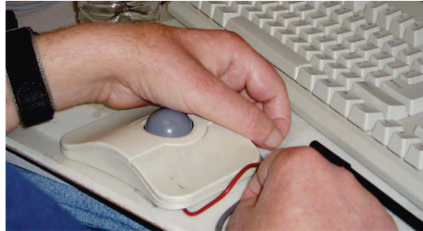
Figure 20. Jim’s favourite trackball is the CoStar Stingray because he can press its wide left button with the palm of his left hand while his left thumb rolls the ball to perform dragging operations, which are traditionally difficult with trackballs.
