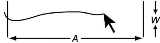
Figure 10. Crossing follows Fitts' law but with the W constraint orthogonal to the movement trajectory, rather than collinear.
